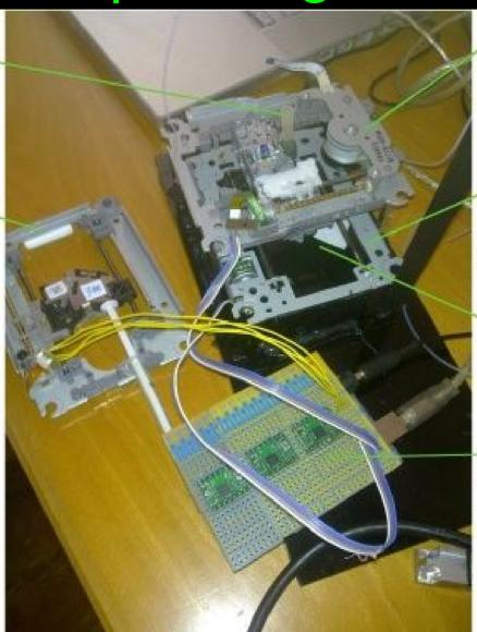
Compact Disc Drive 2 - Drives Dispensing Tip in Y Direction
